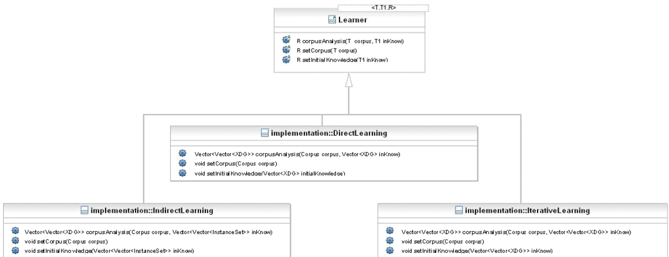
Figure 3: Partial classes diagram of the learning algorithm
