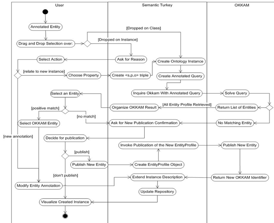
Fig. 2. Entity-centric Annotation Activity Diagram
