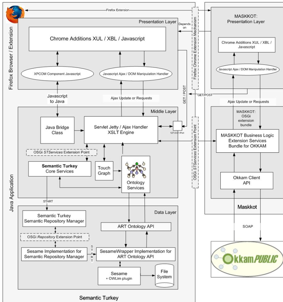
**Fig 4.** Architectural view of the maskkot extension and its interfacing with Semantic Turkey and okkam
